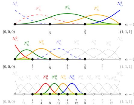
Fig. 1: Basis functions for a three-level quadratic hierarchical spline space, where  $N_i^l$  denotes the  $i$ -th spline function at level  $l$ . Basis functions are indicated by solid colored lines, functions that are linearly dependent on higher-level functions by dashed colored lines, and inactive functions by grey dotted lines. The finite elements correspond to the cells in green.
