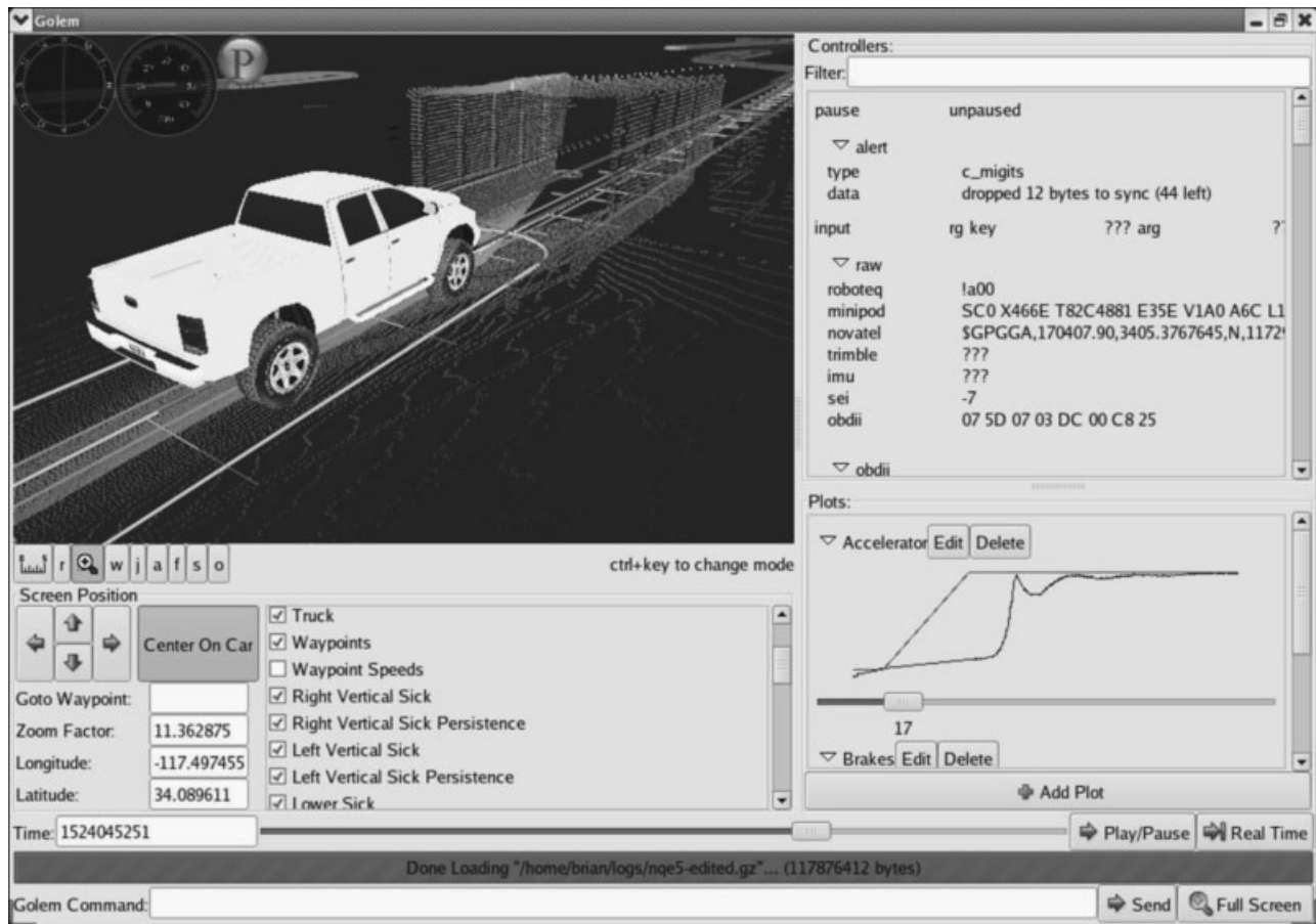
Figure 4. Dashboard visualization of Golem 2 entering a tunnel during an NQE run.
