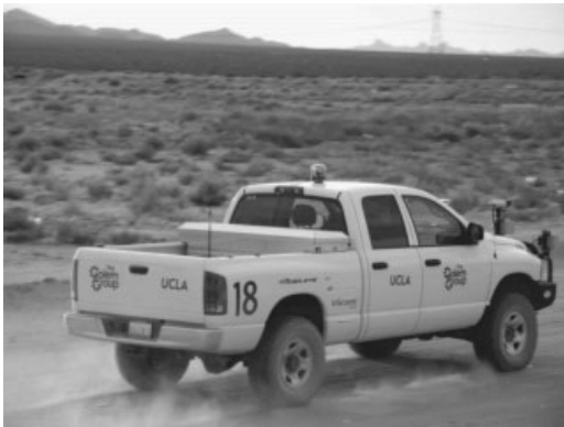
Figure 1. Golem 2 driving autonomously at 30 miles per hour.
