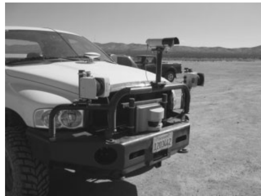
Figure 17. The camera is mounted inside a housing, atop a pole connected to the front bumper. This allows a better field of view than mounting the camera on the windshield.
