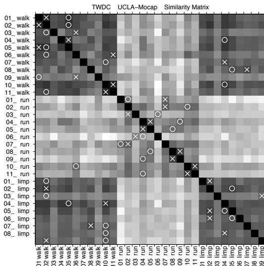
**Fig. 3.** Confusion matrix for the UCLA dataset [10]. There are 31 sequences of (walking, running, limping). Moving along the horizontal axis we mark the first (x) and second (o) nearest neighbors. Classification performance using  $k$  nearest neighbor is reported in the following table.
