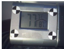
Figure 3. Sample captured temperature sensor image (left), with raw and potentially republished corrected data streams (right). (Data is temperature located on the right bottom of the LCD from 3:22pm to 3:32pm, Feb. 18, 2007.)
