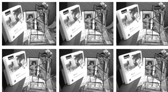
Figure 4. Six images from the original sequence. The estimated normal vectors are shown superimposed to the real scene.
