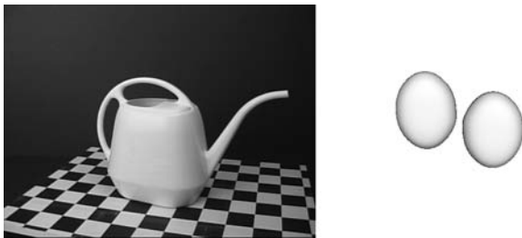
Fig. 9. The “watering can” sequence and the initial surface. In order to capture the surface, it is necessary that the initial surface intersects with the true surface. One way to guarantee this is to start with a number of small surfaces, two in this case.
